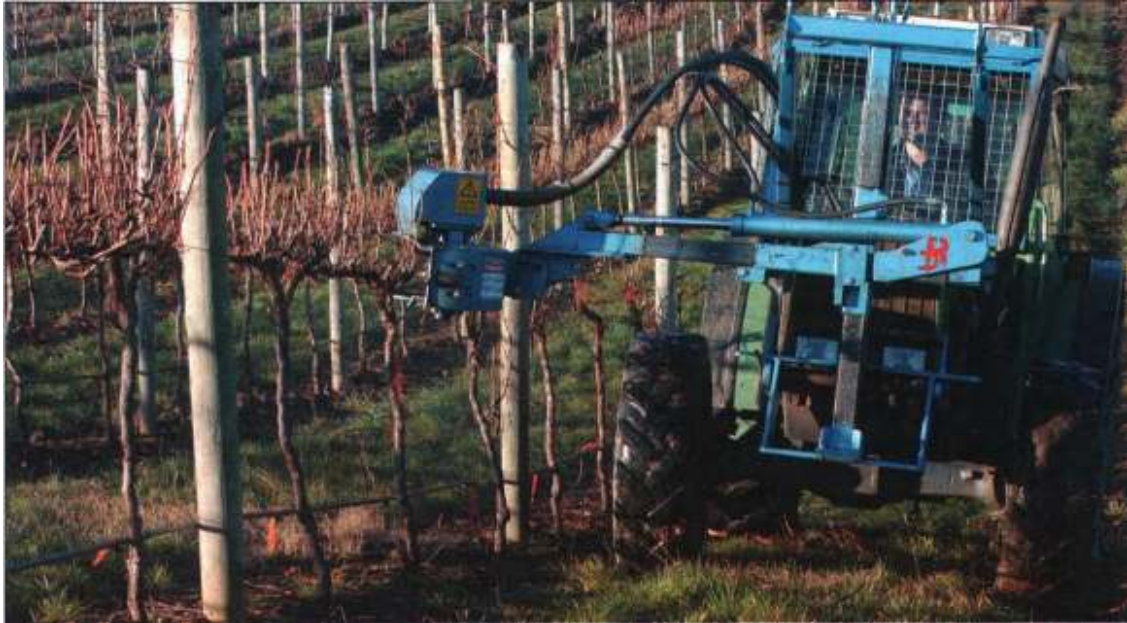
The shredder cuts straight through the vine trunk and removes the cordon without damaging the wire
